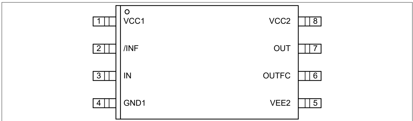
Figure 4 Pinout clamp configuration (top view)
