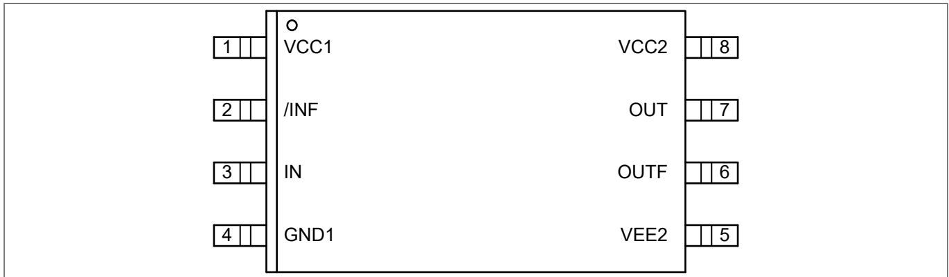
Figure 3 Pinout standard configuration (top view)
