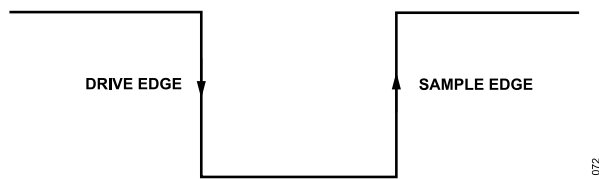
Figure 69. SPI Mode 3, SCLK Edges
