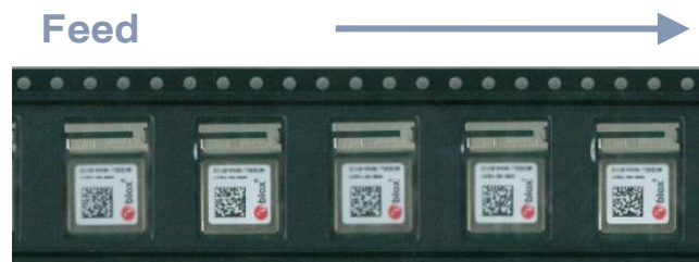
Figure 13: Orientation of NINA-B112 modules on tape
