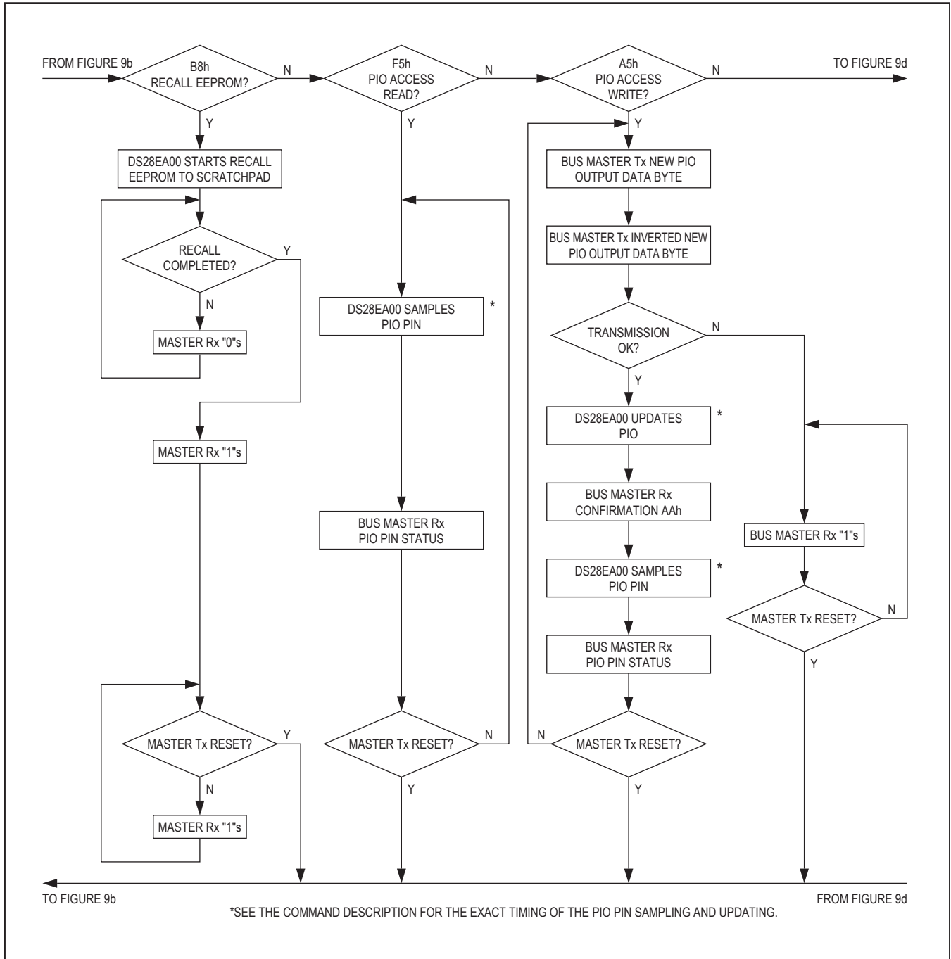
Figure 9c. Control Function Flowchart
