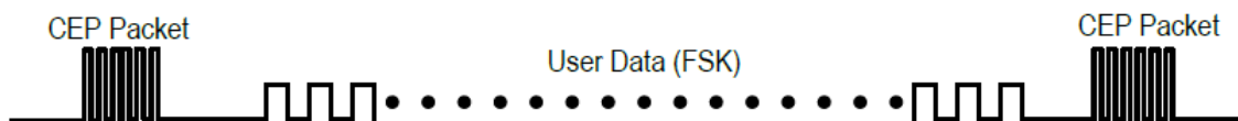
Figure 12. Timing Diagram for the User Data Transfer from the P9235A-RB to the P9222-R
