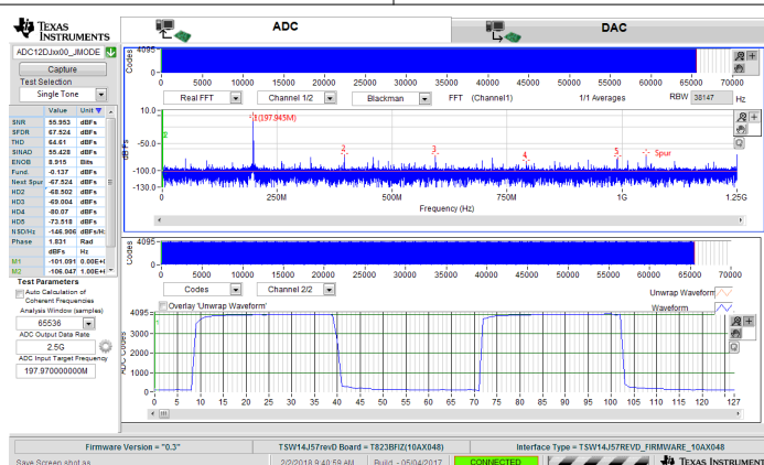
Figure 7-12. 200-MHz, Sine-Wave (Channel A) Frequency Domain (FFT) and 40-MHz, Square-Wave (Channel B) Time Domain for 5-GSPS, Single-Channel Oscilloscope
