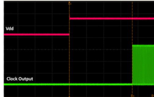
Figure 17. Startup Waveform vs. Vdd
