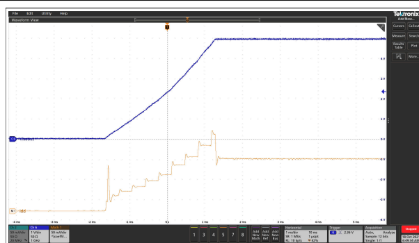
Figure 7-28. Soft Start at 110-mA Load For V_{ISOOUT} = 3.3\text{ V}
