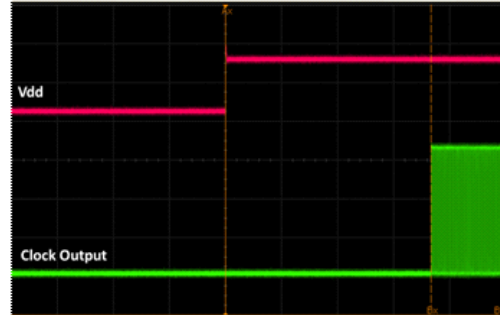
Figure 16. Startup Waveform vs. Vdd
