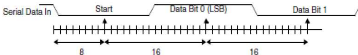
Figure 81: Receiver Serial Data Sampling Points
