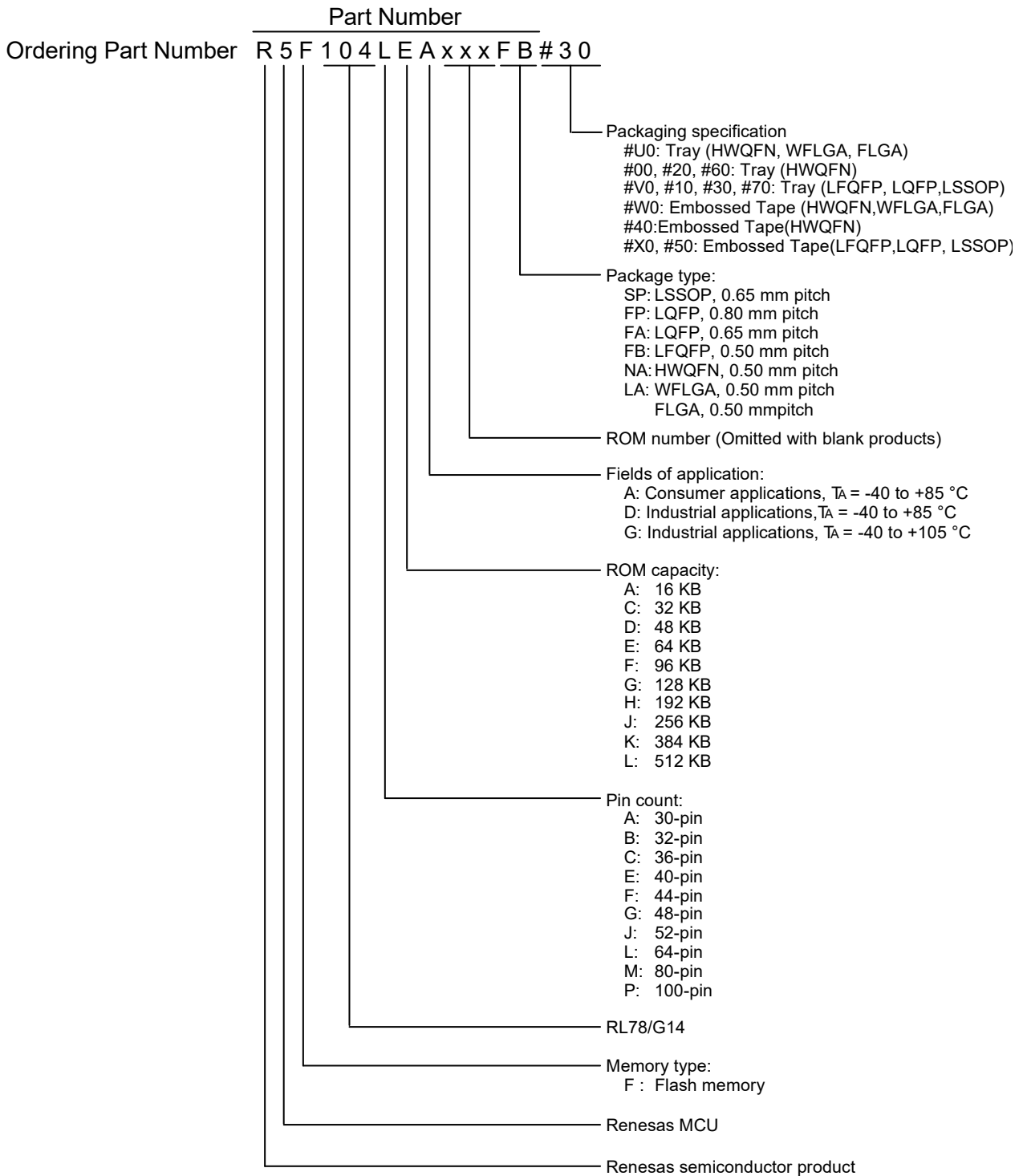
Figure 1 - 1 Part Number, Memory Size, and Package of RL78/G14
