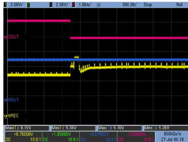
Figure 10. Load Transient: V OUT = 5.5V, 1.2A → 0A
