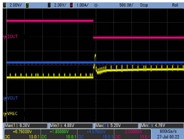
Figure 12. Load Transient: V OUT = 5V, 1.2A → 0A
