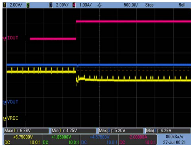
Figure 11. Load Transient: V OUT = 5V, 0A → 1.2A
