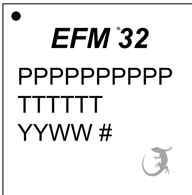
Figure 8.3. QFN40 Package Marking
