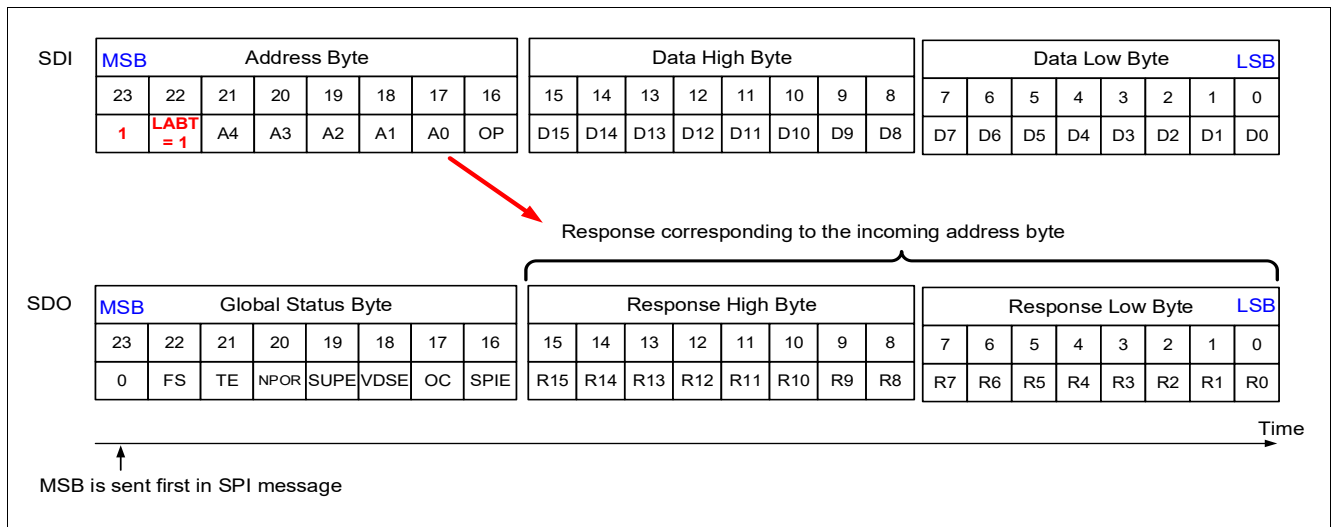
Figure 43 In-frame response with individual slave selection
