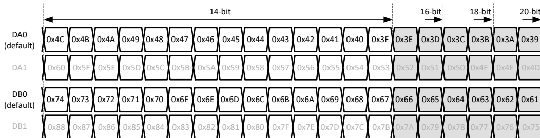
Figure 8-44. 1-wire output bit mapping
