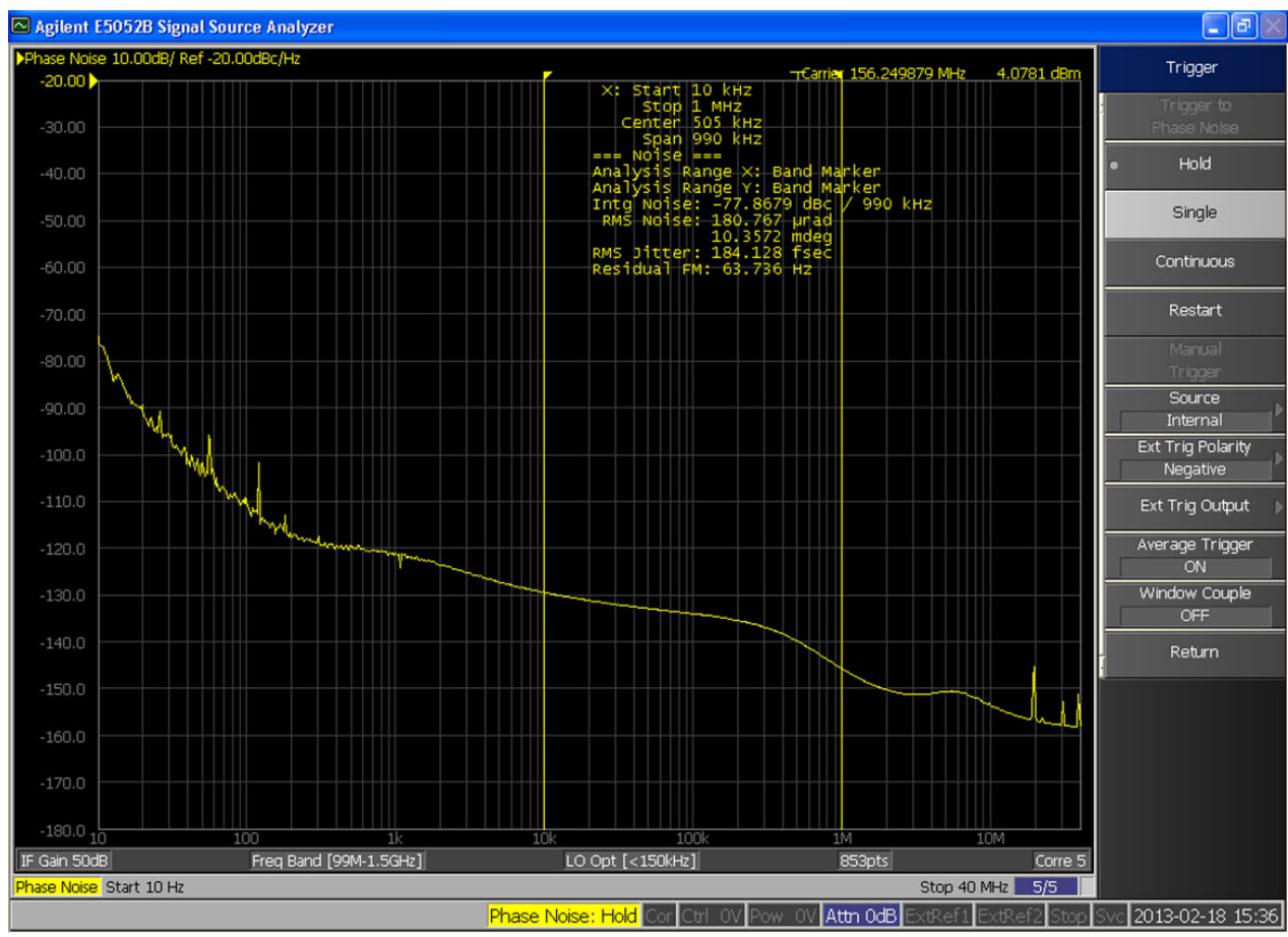
Figure 1. Si535/536 Typical Phase Noise at 156.25 MHz
