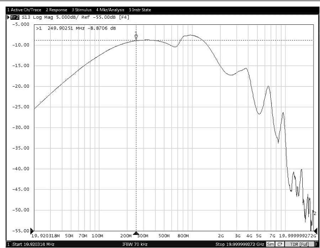
Figure 8-32. Off-State Data-Switch Isolation vs Frequency (TPS25830-Q1)
