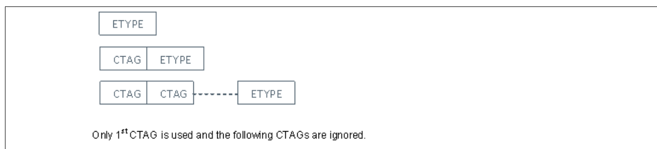
Figure 30 Supported Frame Formats when STAG is disabled
