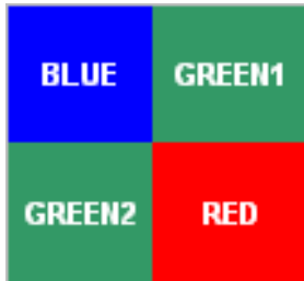
Figure 3. Color Filter Arrangement on the Pixels
