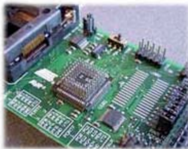
Figure 4-3. Connecting TQFP Adapters (Part One of Three)
