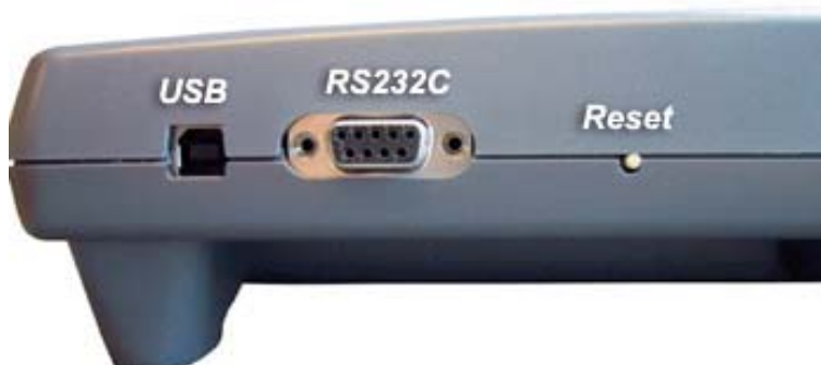
Figure 3-6. USB-, RS-232C-communication, and Reset Button
