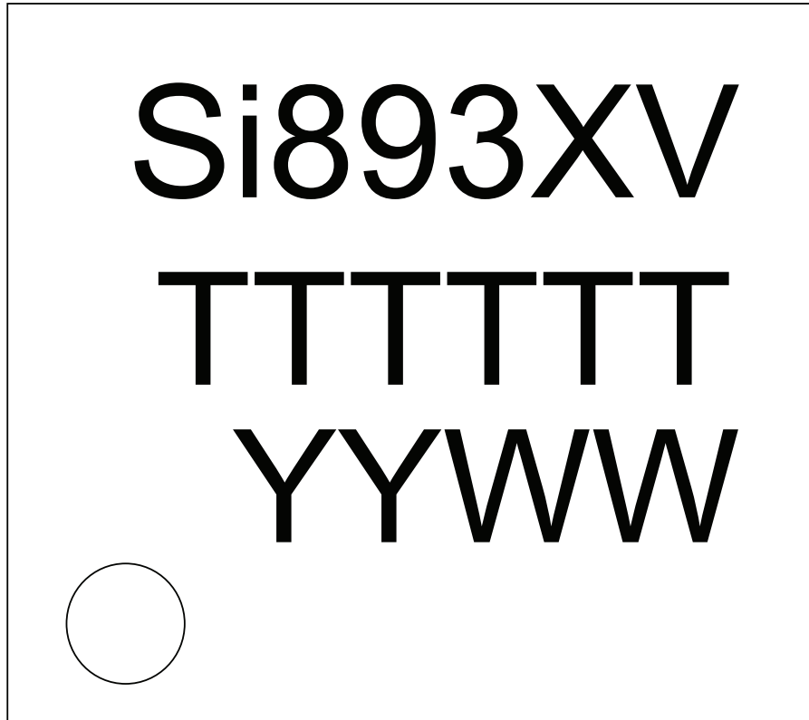
Figure 37. Si8931/32 Typical Package Marking, 8-Pin Wide Body Stretched SOIC
