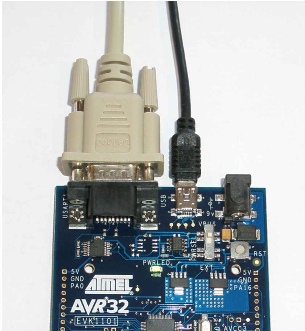
Figure 4-2. Powering the EVK1101 using the USB cable
