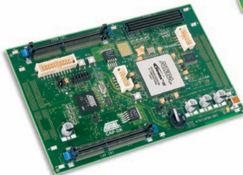
CAP9A Mezzanine Board
