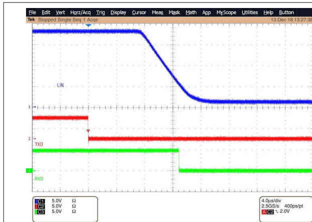
Figure 10-11. Recessive to Dominant Propagation Delay
