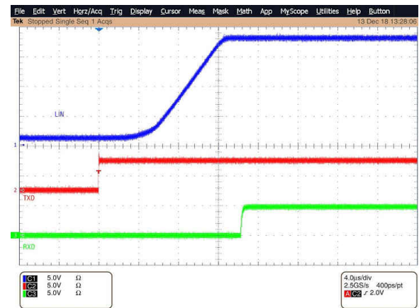
Figure 10-12. Dominant to Recessive Propagation Delay
