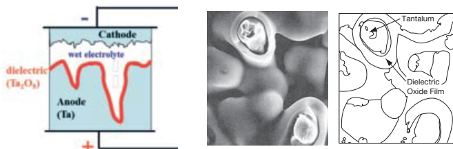
Figure 1 a. Basic Tantalum Wet Electrolytic Capacitor System
