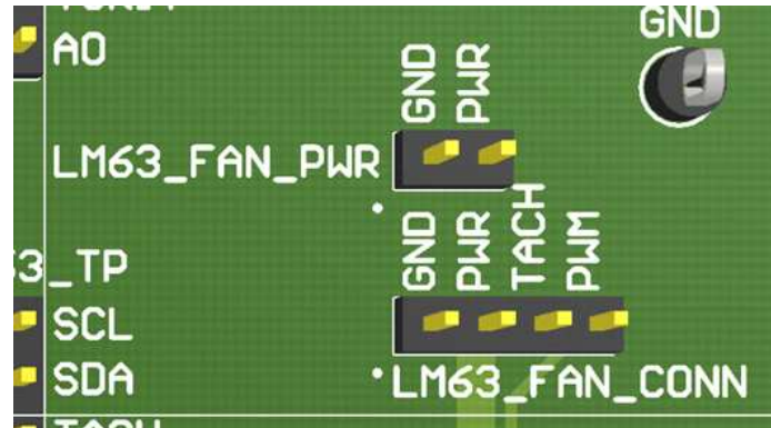
Figure 14. LM63 Fan Connector
