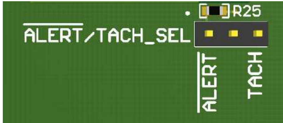
Figure 4. LM63 ALERT/TACH Select Jumper
