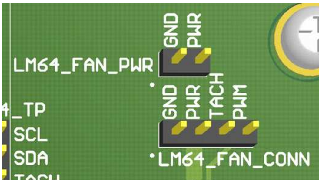
Figure 15. LM64 Fan Connector
