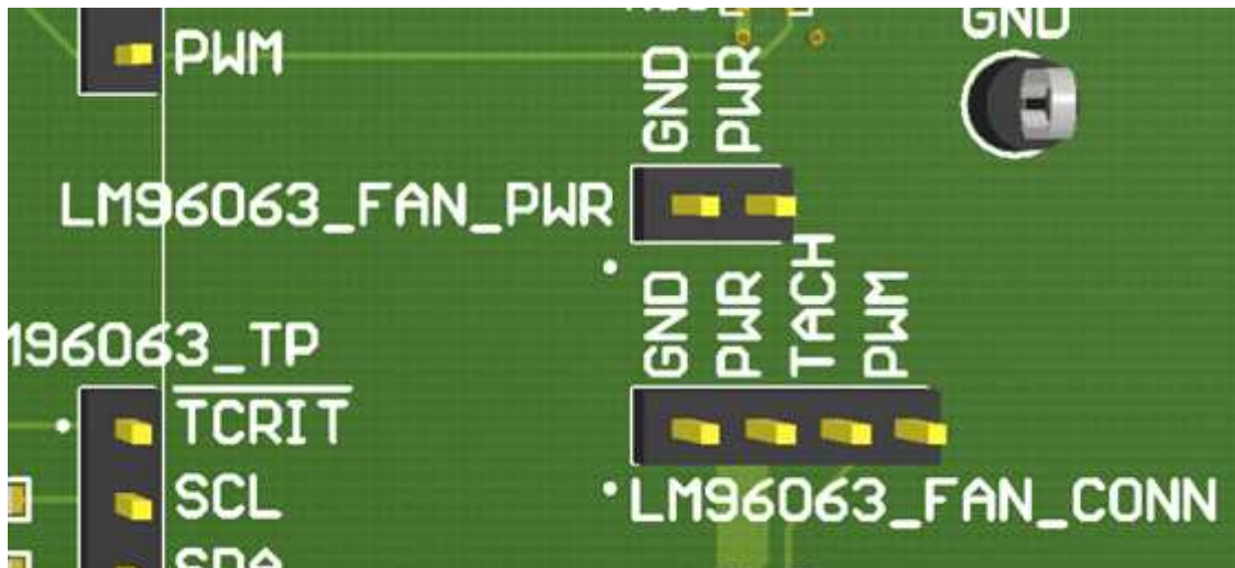
Figure 16. LM96063 Fan Connector
