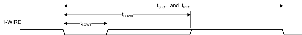
Figure 5-118. 1-Wire Write Bit Timing (Command/Address or Data)
