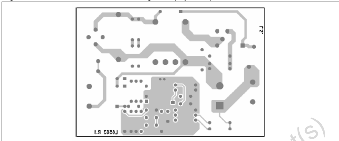
Figure 3. EVAL6563-80W: soldering side (top view)
