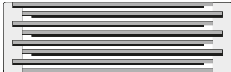
Extended metallized film design
