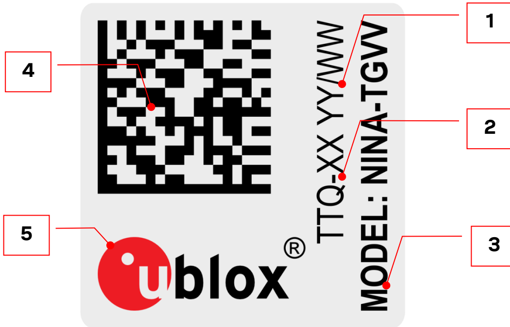
Figure 14: Location of product type number on the NINA-B2 series module label
