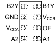
Figure 6-2. DTT Package, 8-Pin SON Transparent (Top View)
