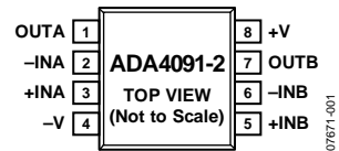
Figure 1. 8-Lead, Narrow-Body SOIC (R-8)
