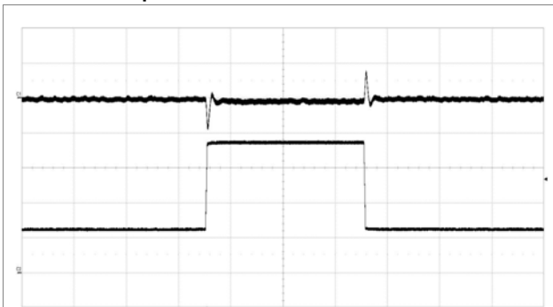
Output voltage response to load current step change (25%–75%–25%) at V_i = 12\text{ V} , C_{OUT} = 2 \times 330\text{ }\mu\text{F}/10\text{ m}\Omega + 6 \times 100\text{ }\mu\text{F} , di/dt = 2\text{ A}/\mu\text{s} , ACSR Gian=200 and ASCR Residual=90. Scale from top: 50 mV/div, 5 A/div, 200 \mu\text{s} /div. Note: Sense pins are connected to load.
