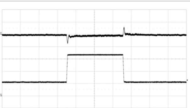
Output voltage response to load current step change (25%–75%–25%) at V_i = 12\text{ V} , C_{OUT} = 4 \times 330\text{ }\mu\text{F}/10\text{ m}\Omega + 12 \times 100\text{ }\mu\text{F} , di/dt = 2\text{ A}/\mu\text{s} , ACSR Gain=200 and ACSR Residual=90. Scale from top: 50 mV/div, 10 A/div, 200 \mu\text{s} /div. Note: Sense pins are connected to load.
