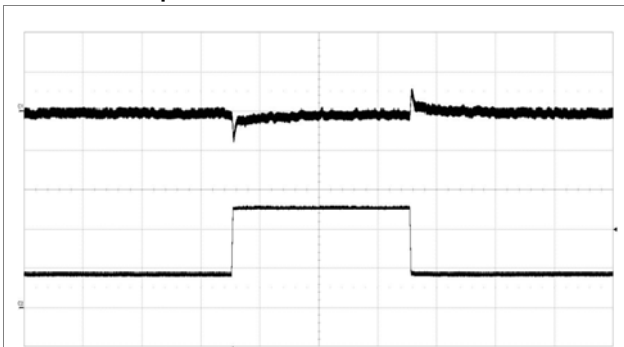
Output voltage response to load current step change (25%–75%–25%) at V_i = 12\text{ V} , C_{OUT} = 2 \times 330\text{ }\mu\text{F}/10\text{ m}\Omega + 6 \times 100\text{ }\mu\text{F} , di/dt = 2\text{ A}/\mu\text{s} , ACSR Gian=200 and ASCR Residual=90. Scale from top: 50 mV/div, 5 A/div, 200 \mu\text{s}/\text{div} . Note: Sense pins are connected to load.
