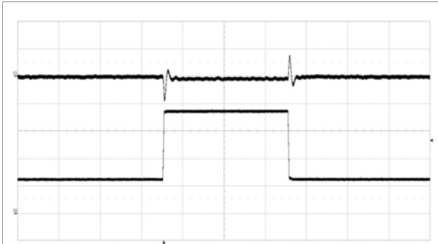
Output voltage response to load current step change (25%–75%–25%) at V_i = 12 V , C_{OUT} = 2 \times 330 \mu\text{F}/10 \text{ m}\Omega + 6 \times 100 \mu\text{F} , di/dt = 2 A/\mu\text{s} , ACSR Gian=200 and ASCR Residual=90. Scale from top: 50 mV/div, 5 A/div, 200 \mu\text{s}/\text{div} . Note: Sense pins are connected to load.
