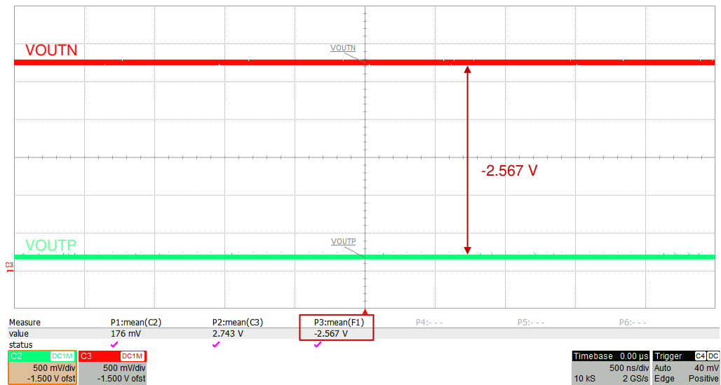
Figure 7-5. Typical Fail-Safe Output of the AMC3330
