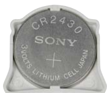
Insert Coin Cell into the Tray
