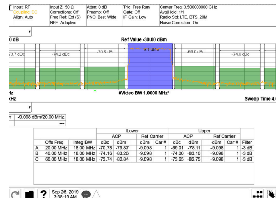
Figure 6-137. TX IMD3 vs DSA Setting at 3.5 GHz
