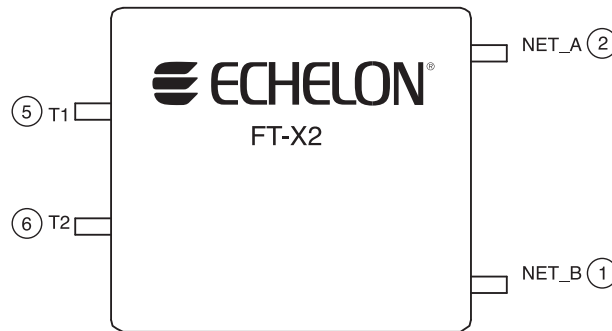
4-pin surface mount transformer (top view)
