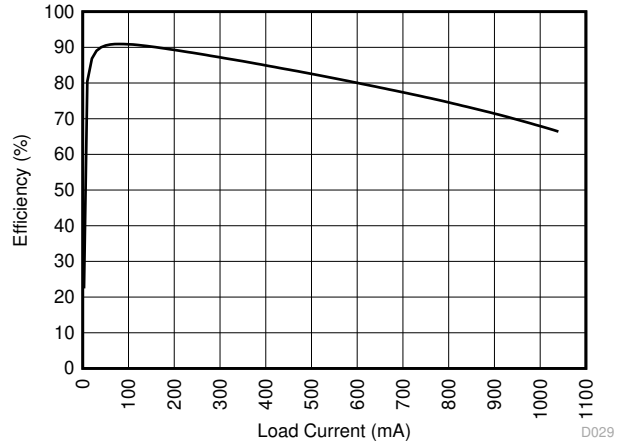
SN6505A-Q1 + Würth 750316031 V_{CC} = 3.3\text{ V}
