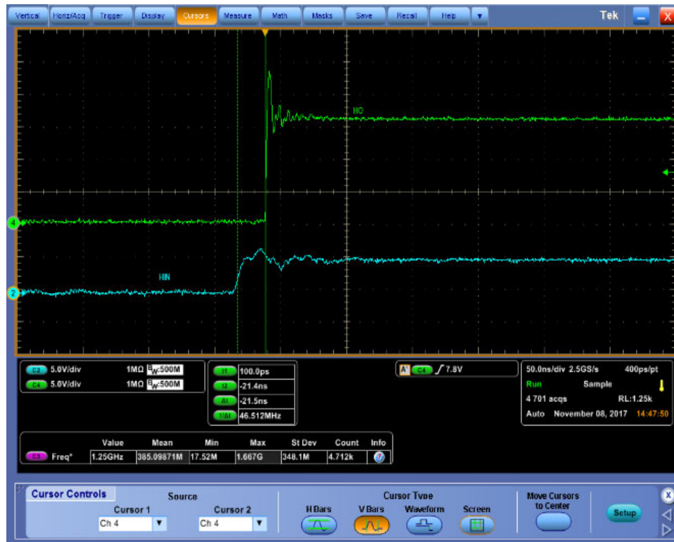
Figure 31. High Side Turn-Off Propagation Delay (NCP51530B)
