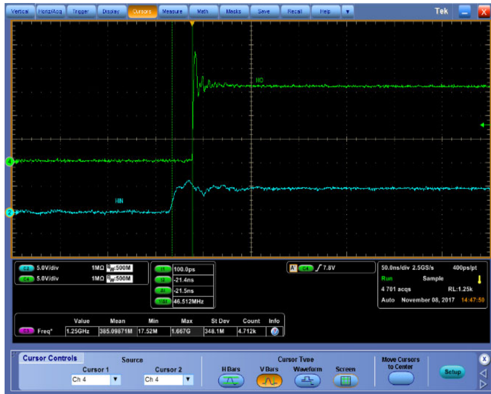
Figure 31. High Side Turn-Off Propagation Delay (NCP51530B)
