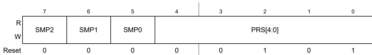
Figure 15-7. ATD Control Register 4 (ATDCTL4)
