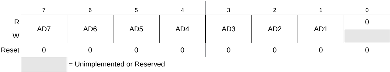
Figure 11-3. IIC Address Register (IICxA)
