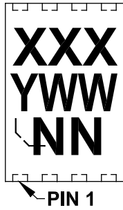
8-Lead DFN (2x3) (MCP4011)
