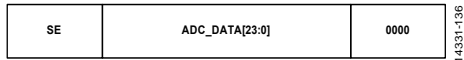
Figure 36. Format for the ADC Data Stored in the Waveform Buffer, x\_SINC\_DAT and x\_LPF\_DAT Registers
