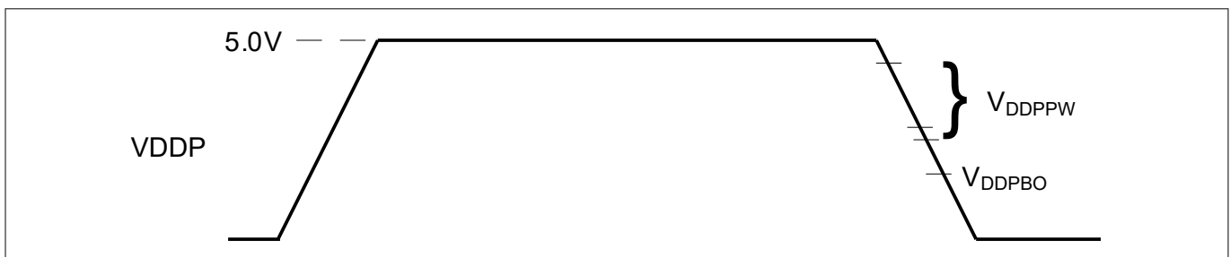
Figure 17 Supply Threshold Parameters
