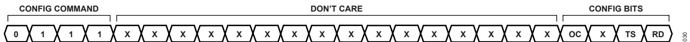
Figure 34. Configuration Command Syntax, Open-Circuit (OC) Detection Disable, Thermal Shutdown (TS) Disable, and Reference Disable (RD)
