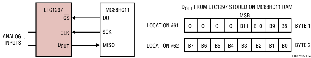
Figure 4. Hardware and Software Interface to Motorola MC68HC11 Microcontroller
