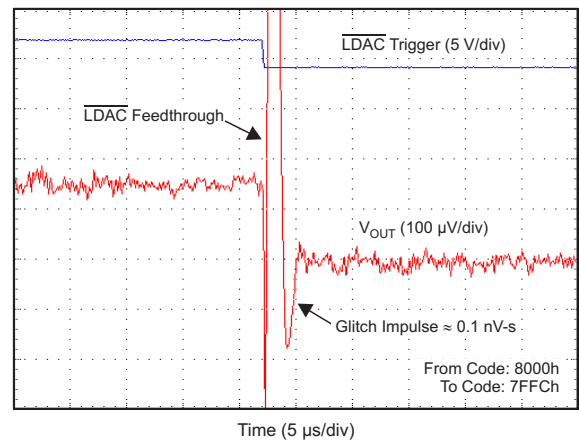
Figure 80. Glitch Impulse, Falling Edge, 1-LSB Step
