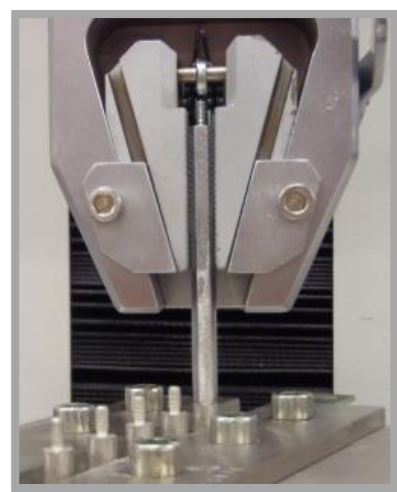
Checking fixture Pull Strength
