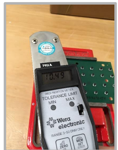
Digital torque wrench for Breaking Torque
