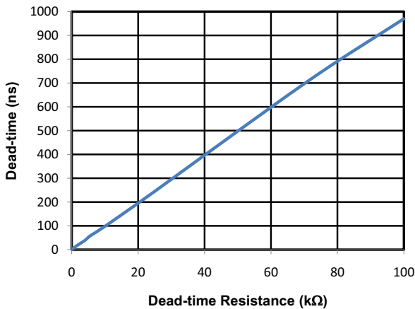
Figure 37. Dead Time vs. Resistance ( R_{DT} )
